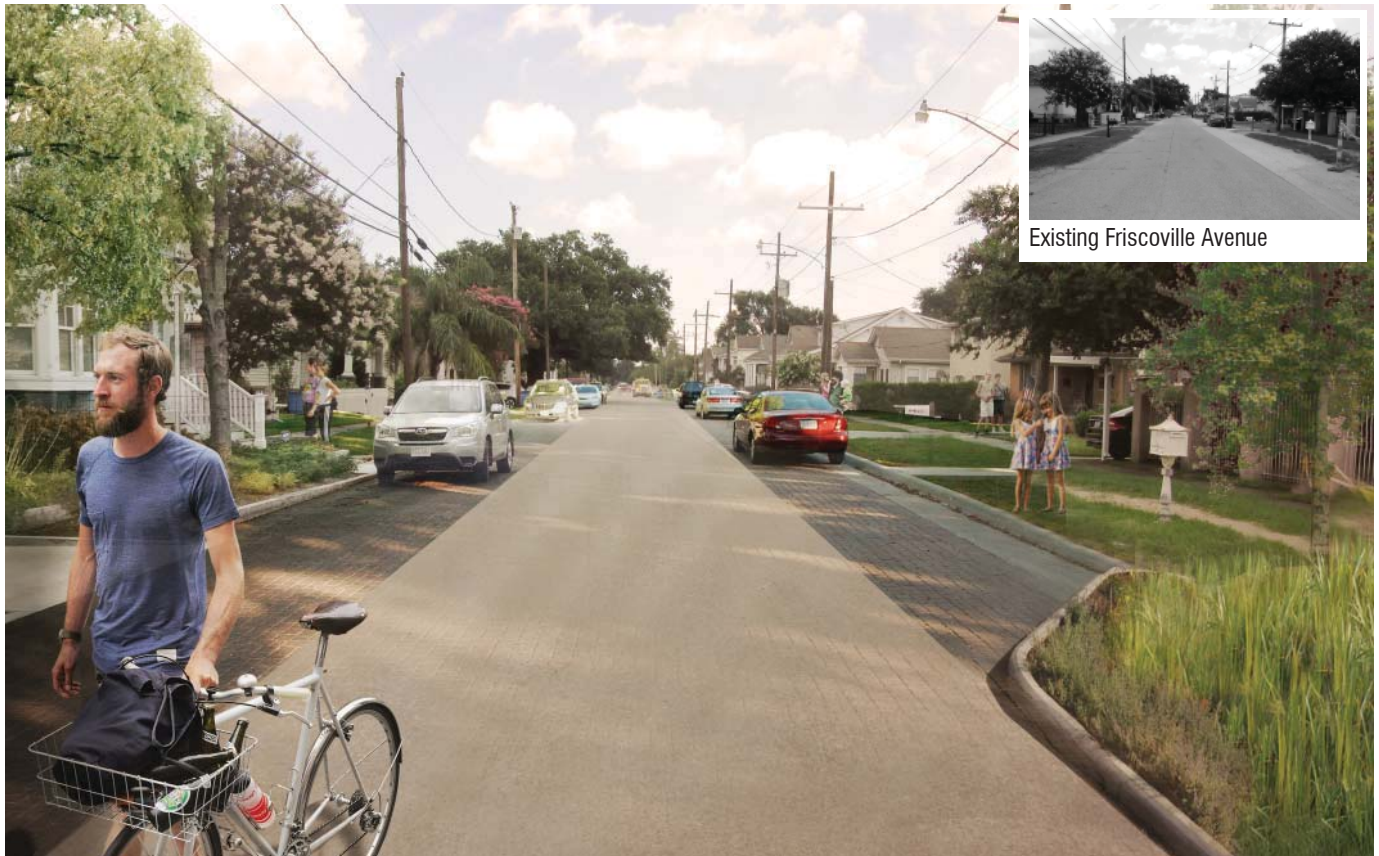
Proposed Friscoville Avenue, with bump outs for rain gardens that also define pervious paving lanes for parking
