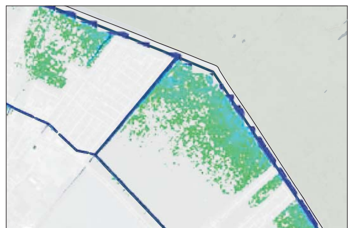
Below: Option 4 Intensive shows that spillways and weirs hold water
