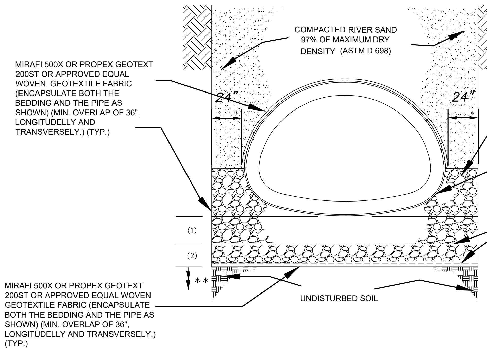
TYPICAL CONCRETE DRAINAGE PIPE TRENCH DETAIL
