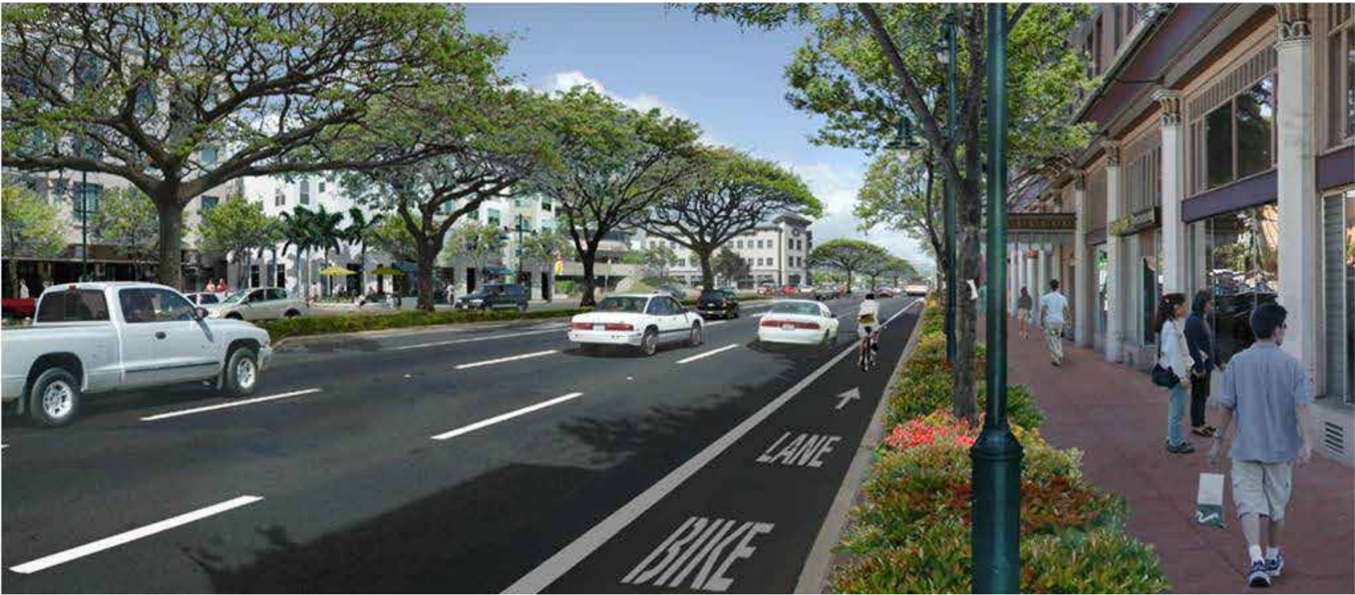
Figure 65: Complete Streets are those that include adequate facilities for automobiles (road travel lanes), bicycles (bicycle lanes, trails/paths, and/or shared vehicle travel lanes), and pedestrians (sidewalks and/or shared trails/paths). (image courtesy of Urban Advantage)
